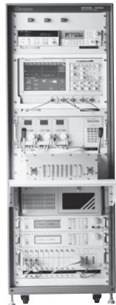
DC to DC Converter ATS
